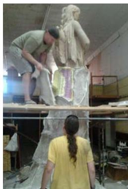
Omega Bronze Foundry takes molds from the clay Angel, sculpted by Bill McGlaun.
